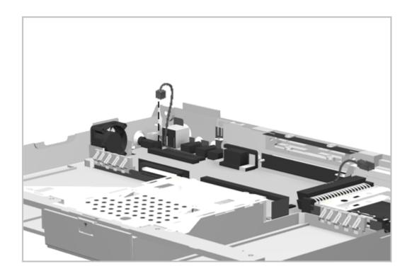
Figure 5-54. Removing the Microphone Extension Cable
